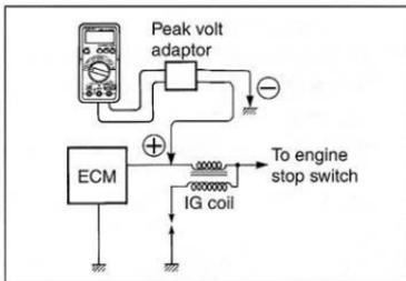
If the peak voltage is lower than the standard range, check the peak voltage at the ECM coupler.
