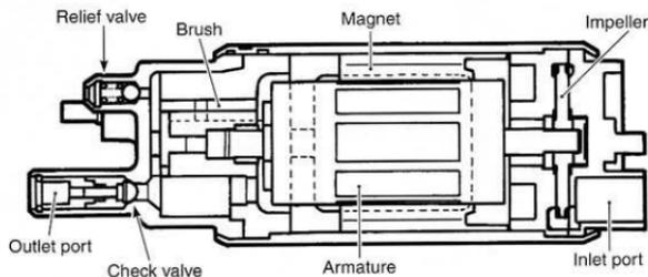
When the impeller is driven by the motor, pressure differential occurs between the front part and the rear part of the blade groove as viewed in angular direction due to fluid friction. This process continuously takes place causing fuel pressure to be built up. The pressurized fuel is then let out from the pump chamber and discharged through the motor section and the check valve.
