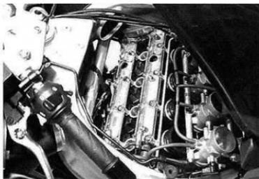
The tappet clearance specification is different for intake and exhaust valves.
