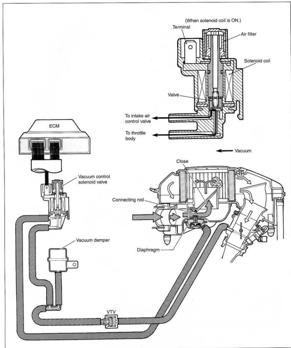
When the engine is running in a medium to high speed range, the signal from the ECM discontinues. Then, the solenoid coil is de-energized, causing vacuum on the throttle body side to stop being transmitted to the intake air control valve side. At the same time, the vacuum control solenoid valve let atmospheric pressure into the diaphragm side vacuum line, which deactivates the diaphragm and allows the spring to return and open the intake air control valve through the connecting rod.
