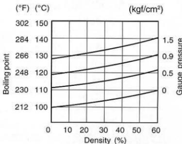
Fig.2 Engine coolant density-boiling point curve.
