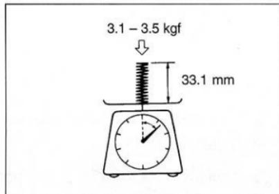
**VALVE AND VALVE SPRING REASSEMBLY**
