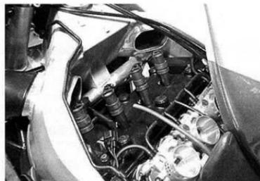
Inspect each ignition coil primary peak voltage at the ignition coil/plug cap coupler.
