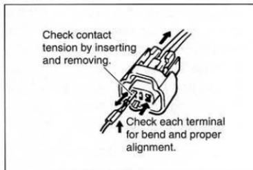
If contact tension is not enough, rectify the contact to increase tension or replace.
