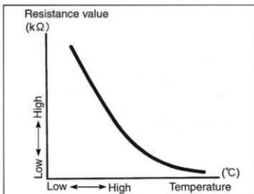
**ENGINE COOLANT TEMPERATURE SENSOR (ECT SENSOR)**
