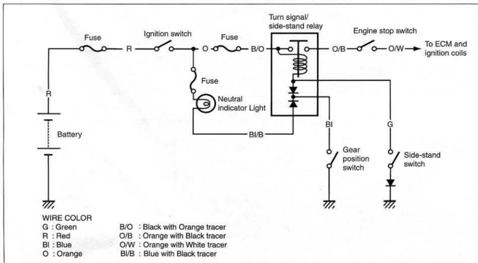
The circuit consists of the turn signal/side-stand relay, neutral indicator light, gear position switch and side-stand switch. The ignition coils will send voltage to the spark plugs dependant on what gear the transmission is in and whether the side-stand is either up or down. The gear position and side-stand switches work together in this system. The ignition coils work only in two situations as follows.
