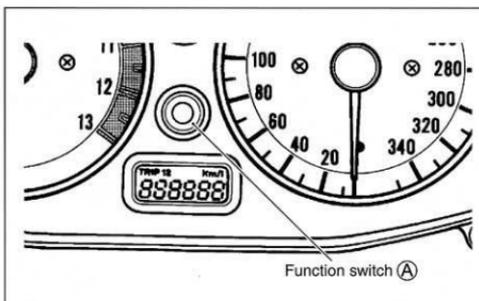
Pointer will return to the starting point right after the completion of the operation. In the case of the pointer not returning to the proper position after doing above, replace the combination meter unit.
