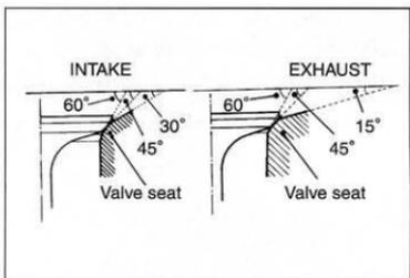
**TOOL 09916-21111: Valve seat cutter set****09916-22420: Valve seat cutter (N-114)****09916-22430: Valve seat cutter (N-128)****09916-24311: Solid pilot (N-100-5.0)****NOTE:**
