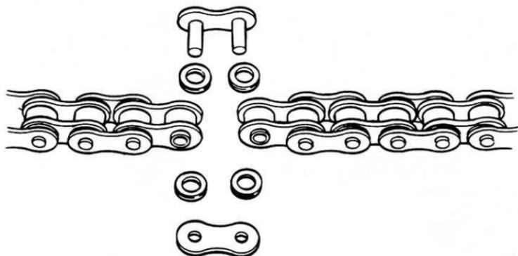
Use the special tool in the following procedures, to cut and re-join the drive chain.
